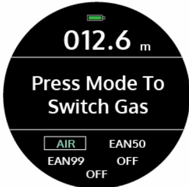
Tec Mode - Gas Switch (Before switching)
