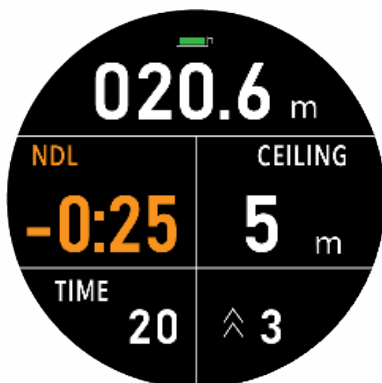
Scuba Mode – Underwater When the NDL has been exceeded (first three minutes)
