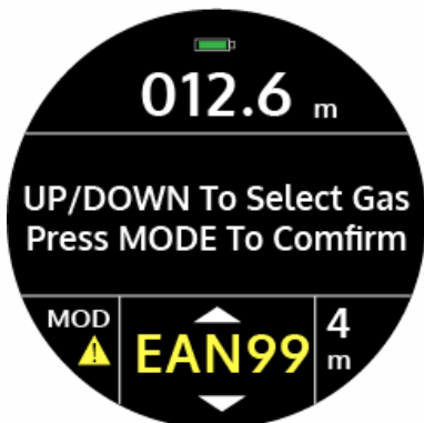
Tec Mode - Gas Switch (Current depth exceeds the MOD of the selected gas)
