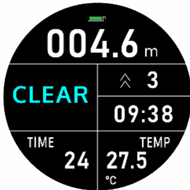
Scuba Mode – Safety stop finished (When the NDL has not been exceeded)
