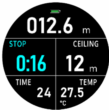
Scuba Mode – Underwater When exceeding the NDL and ascent to ceiling depth.
